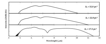
**Fig. 1:** Spectral profiles of sech-Gaussian pulses at the end of 1.38 μm long SQW nanostructure, for three different values of control Rabi frequencies  $\Omega c = 32.0$  ps-1 (top),  $\Omega c = 22.0$  ps-1 (middle), and  $\Omega c = 17.5$  ps-1 (bottom). Pulse peak power 400 W and FWHM pulse duration 50 fs.
